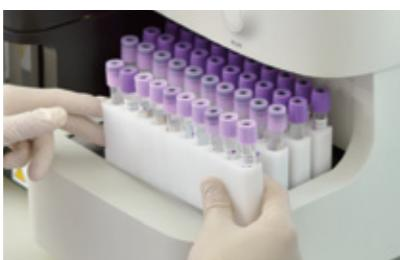
Loading up to 60 samples simultaneously, it tests up to 80T/H, which enhances efficiency greatly.
